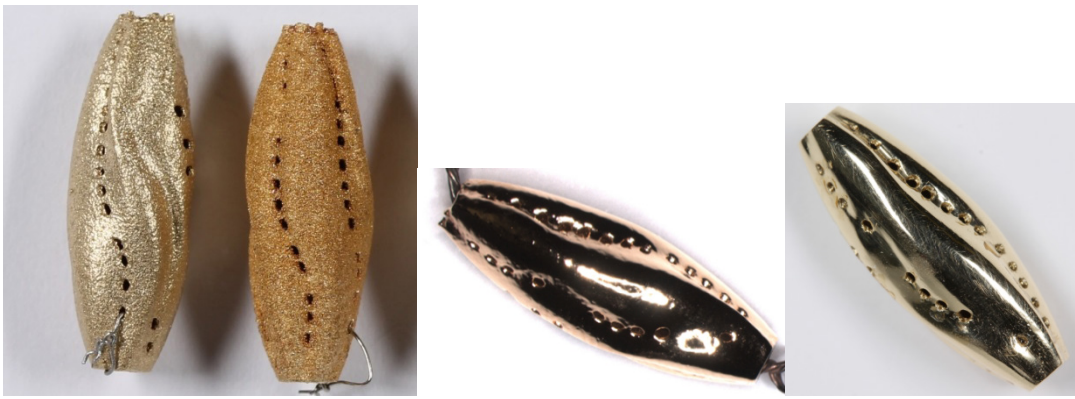
Figure 20: Jewelry samples in standard yellow gold in the different polishing steps. From left to right: as-manufactured, sand blasted, electro polished, hand polished
