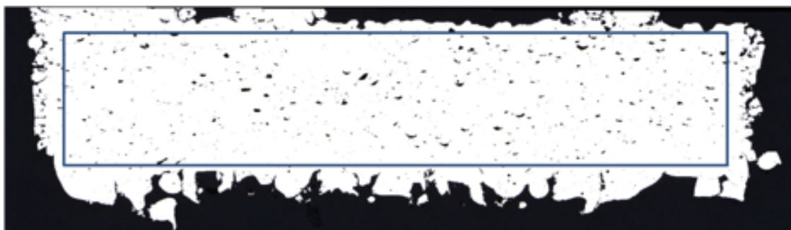
Figure 7: Rectangular area for porosity determination by optical microscopy and image analysis
