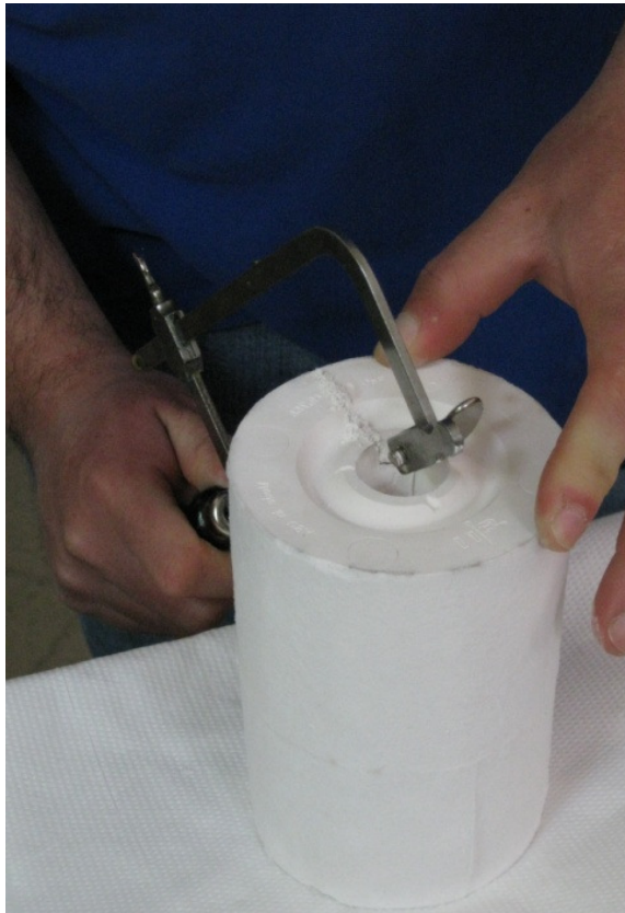
Fig. 15 Opening the coating after calcination (a). An example of a cavity (b).
