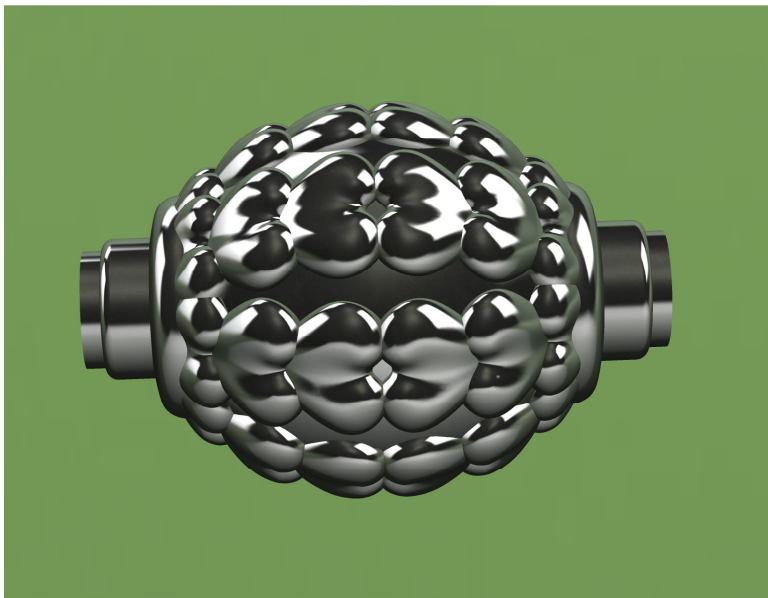
Figure 20. The master model for the casting pattern must have the core included with the locating features.
