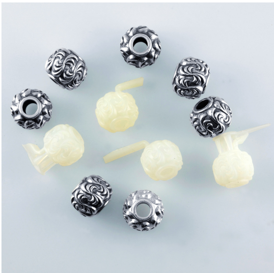
Figure 18. SLA-grown resin pattern for direct casting
