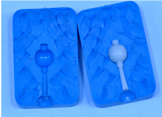
Figure 21. Water-soluble wax core.
