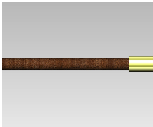
Figure 7. Wax sheet wrapped on mandrel
